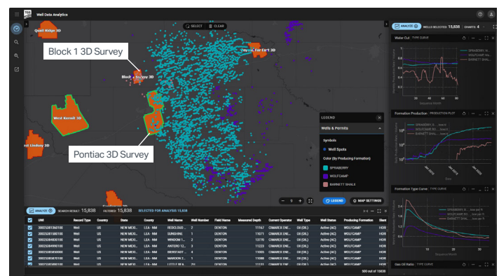
Figure 1. TGS Well Data Analytics application displays active producing Barnett, Spraberry and Wolfcamp wells in the Midland Basin, overlaying with 3D Seismic Surveys and accompanying production plot, water cut and type curves.
