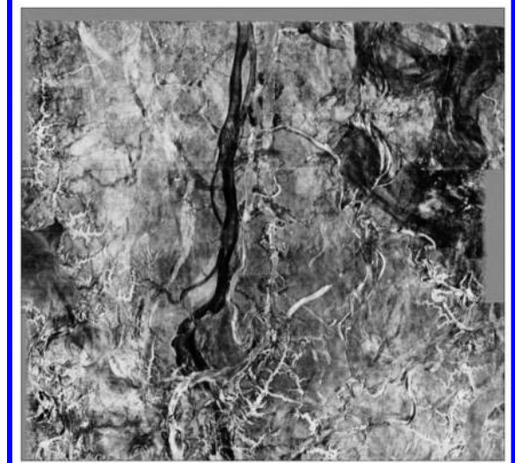
Figure 3: Shallow water survey (ca. 70m) offshore Malaysia (courtesy Lundin). The SWIM image at 105m depth (bottom) has accurately filled in the holes caused by refraction when only primaries are used (top). The spread was made of 12 multi-component streamers 75m apart.
