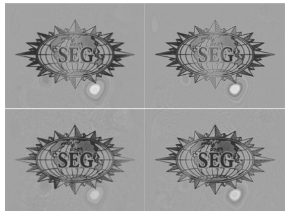
Figure 4: Depth migrated images of the SEG logo: primaries WEM (top-left), primaries RTM (top-right), SWIM WEM (bottom-left), and SWIM RTM (bottom-right).
