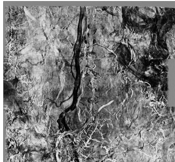
Figure 6 depth slices at 105 meters from imaging of primaries (top) and multiples (bottom). Multiples very well mitigate the acquisition footprint and generate very high resolution 3D depth images, which could be useful to reduce well drilling geohazard risks.
