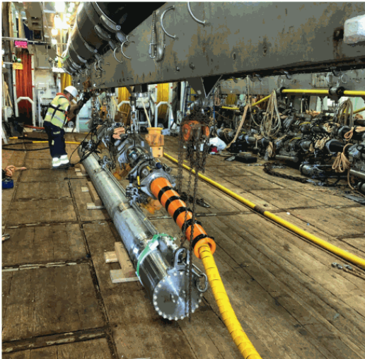
Figure 5. 26 500 in 3 TPS below a conventional air gun source array float. From Tellier et al. (2021) , Figure 2.
