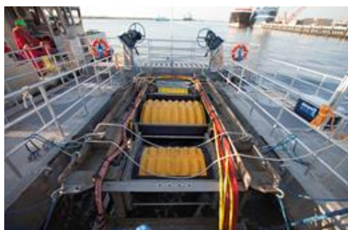
Figure 8. SAExploration marine vibrator array. Refer also to Pramik et al. (2015) .
