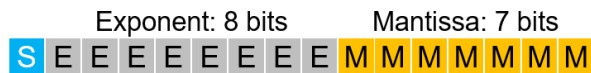
Figure 3. Schematic comparison of 32-bit IEEE floating point format, 16 bit IEEE floating point format, and the new 'brain' floating point format used for TPU chips.
