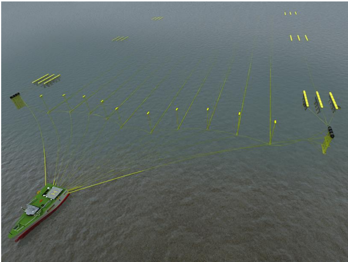
Figure 7. Conceptual towing of marine vibrator arrays by the streamer vessel. Each marine vibrator unit would have a low power and telemetry connection to the vessel, but no air supply requirement.
