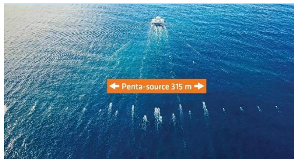
Figure 2: Drone picture showing the ultra-wide penta source configuration with 78.75 m source separation and 315 m total source separation, in combination with a high density 16-streamer spread. Note that the source separation is significantly wider than the streamer separation. For practical reasons, the center source consisted of two source sub arrays.
