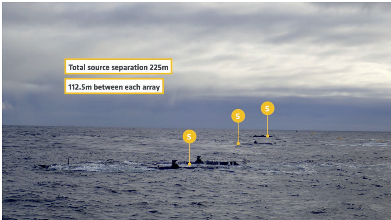
The Viking Graben survey used the widest-ever source separation towed by a single streamer vessel on a commercial project.
