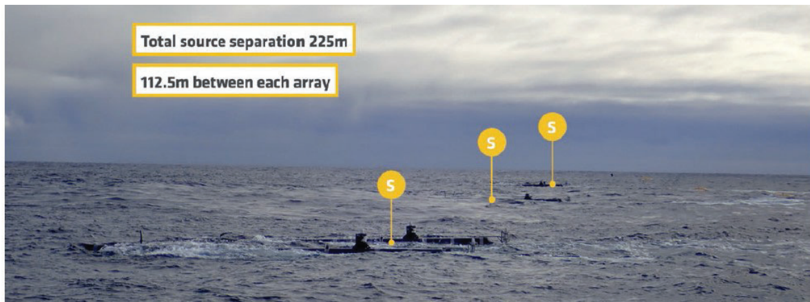
Figure 1 The multi-azimuth acquisition project in the Viking Graben used the widest source separation towed by a single streamer vessel on a commercial project to date.
