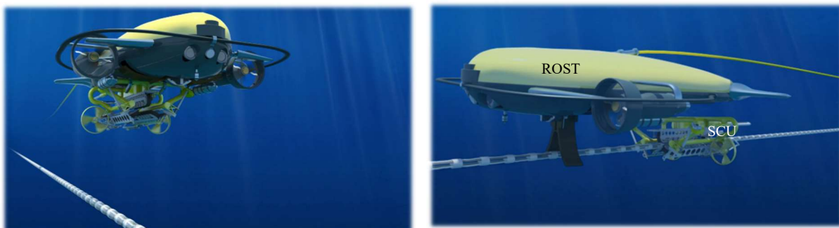
Figure 1: Landing on the streamer (left). The vehicle after having deployed a SCU on the streamer (right).
