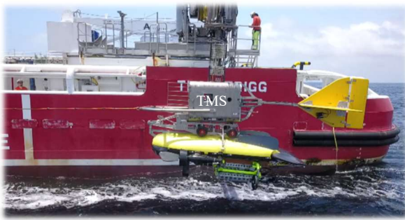
Figure 2: A) The ROST deployed off the side of a support vessel while latched into a TMS (left), and B) Support vessel positioned over the streamer front while the vehicle is deployed.
