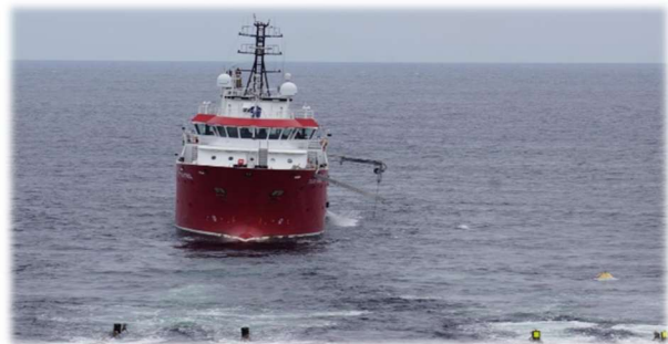
Figure 2: A) The ROST deployed off the side of a support vessel while latched into a TMS (left), and B) Support vessel positioned over the streamer front while the vehicle is deployed.
