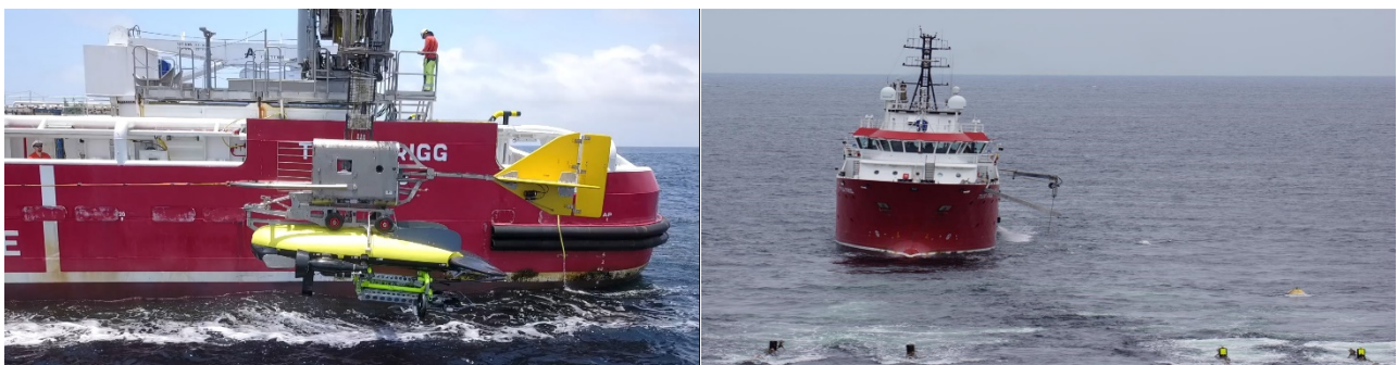
Figure 2. (left) The ROST deployed off the side of a support vessel while latched into a TMS; and (right) Support vessel positioned over the streamer front while the ROST is deployed.
