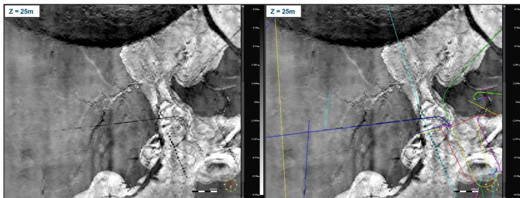
Figure 2 Shallow (25 m depth) image offshore GoM, near Louisiana / Texas border. This 60 Hz SWIM image clearly shows Sabine River outflow and deltaic system. Pipelines present at time of acquisition are also visible. Left: SWIM image. Right: the same SWIM image with pipelines overlaid.
