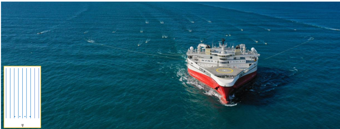
Figure 3: Ramform Hyperion acquiring a high-resolution CCS baseline survey for the Northern Endurance Partnership offshore UK in 2022. The configuration consisted of 11 multisensor streamers with 50m separation and a wide quad source that was towed over the front end of the streamer spread. The resulting nominal acquisition bin size was 6.25m x 6.25m.
