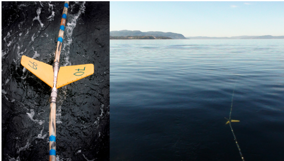
Figure 3 Picture from one of the qualification tests of dual-/multi-sensor streamer steering. The inline design of the steering device produces less towing noise than conventional birds (Hillesund et al. , 2012).
