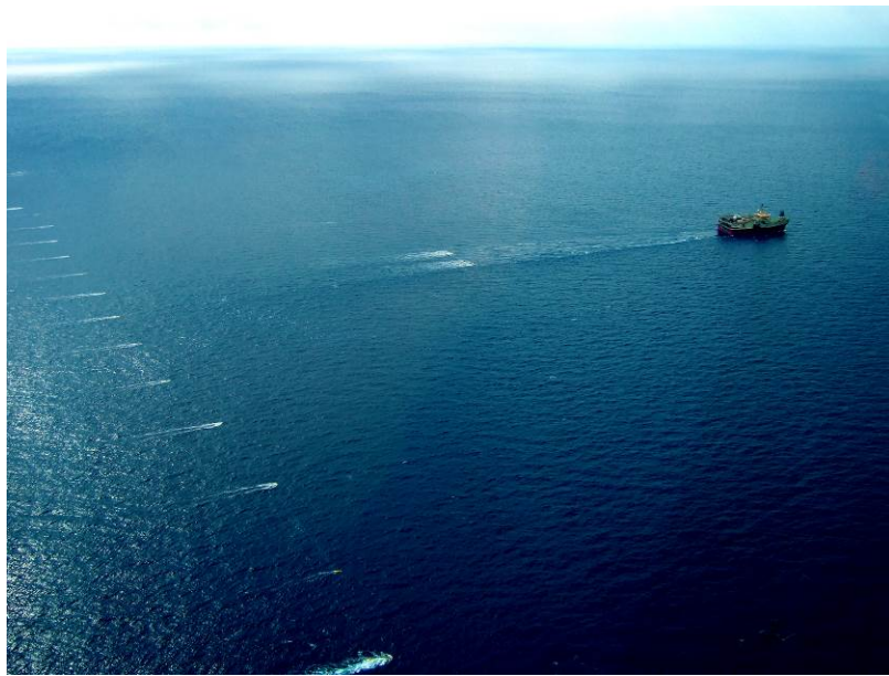
Figure 1 Cost effective single vessel narrow azimuth acquisition is the most frequently used 3D seismic survey method with towed streamer technology.
