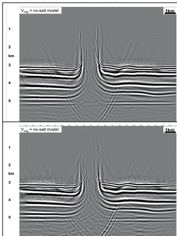
Figures 5 & 6. RTM images of the raw data and the data processed with ASMA and Tau-P muting. The overturned salt wall reflectors have been significantly damaged by this conventional pre-processing flow.
