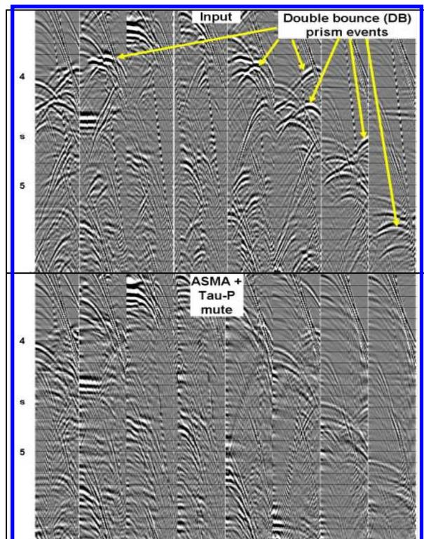
Figures 3 (top) & 4 (bottom): selection of CMP gathers from the FD modeled data, showing the raw input, and the output from an Apex Shifted Multiple Attenuation scheme (ASMA) plus Tau-P muting. Apex shifted events are ‘successfully’ attenuated.
