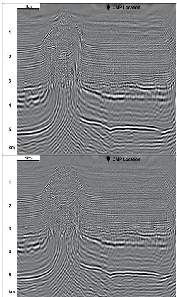
Figure 8. Top: 2D RTM of real data (after SRME multiple suppression) using a 'no salt' model. We see double bounce energy arrivals appearing as near-vertical events primarily in the vicinity of the right hand salt flank. Bottom: 2D RTM with the same model, but using as input the data after the Tau-P mute. The suspected double bounce energy has been removed. The surface location of the CMP shown in Figure 7 is indicated.
