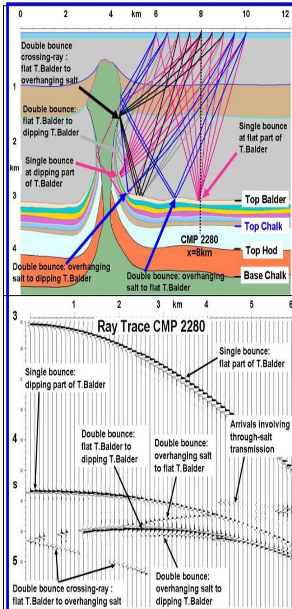
Figure 1 (top), plot of a few sparse rays shown against the interval velocity model. The absence of a strong sediment gradient precludes turning rays in the sediments, although a strong compaction velocity gradient below the Top Balder and top Chalk does produce turning rays. A single CMP gather (from the surface location at 8km) is shown in figure 2 (bottom).
