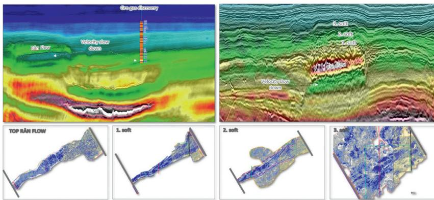
**Figure 6** The Rån volcanic flow may have created traps above and below by sinking into soft Paleogene sediments north in the Vøring Basin. Four potentially prospective levels have been identified based on DM-FWI velocity (top left) and seismic amplitudes (four boxes below). The slower velocity observed under the Rån Flow is like the slow velocity anomaly in the Gro gas discovery beside.
