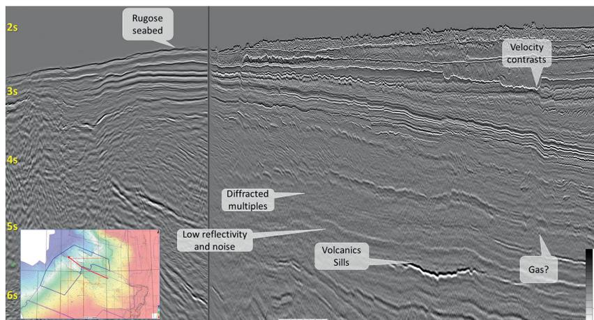
**Figure 1** shows some of the processing challenges encountered in the Atlantic Margin, with 2D seismic on the left, and triple source, 3D seismic with original time processing on the right.
