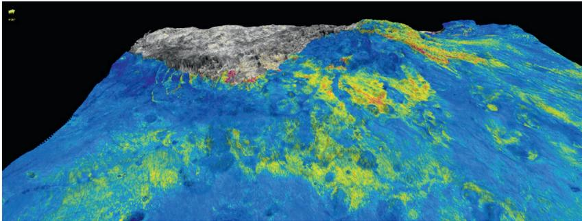
**Figure 4** shows the top basalt and outcropping Kolga High granites within the grey area and, in warm colours, the rms amplitude anomalies of deltas, presumed quartz-rich sands coming from Kolga High. There are no wells yet in this 15000 km<sup>2</sup> 3D area covered by seismic.
