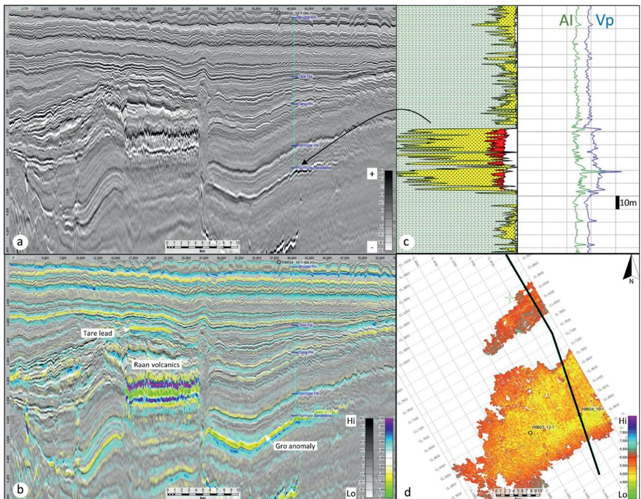
**Figure 3** a) NNW-SSE seismic stack section intersecting well N6604/10-1, b) rEEI<sub>27</sub> inversion showing the Gro rEEI anomaly and an rEEI generated lead in the Tare Formation above the Rån volcanics, c) petrophysical interpretation from the N6604/10-1 well showing gas in the Cretaceous age, Springar Sandstone and the p-wave velocity and acoustic impedance characteristics of the seal and reservoir, d) extent of visible Springar Sand gas anomaly (yellow) and line of section.
