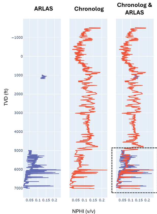
Figure 6: Log track comparison between synthetic logs (red) and ARLAS (blue) for a selected well.
